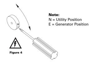
Manual operation is possible for maintenance purposes only. Manual operation of the switch can be checked before it is operated electrically.
